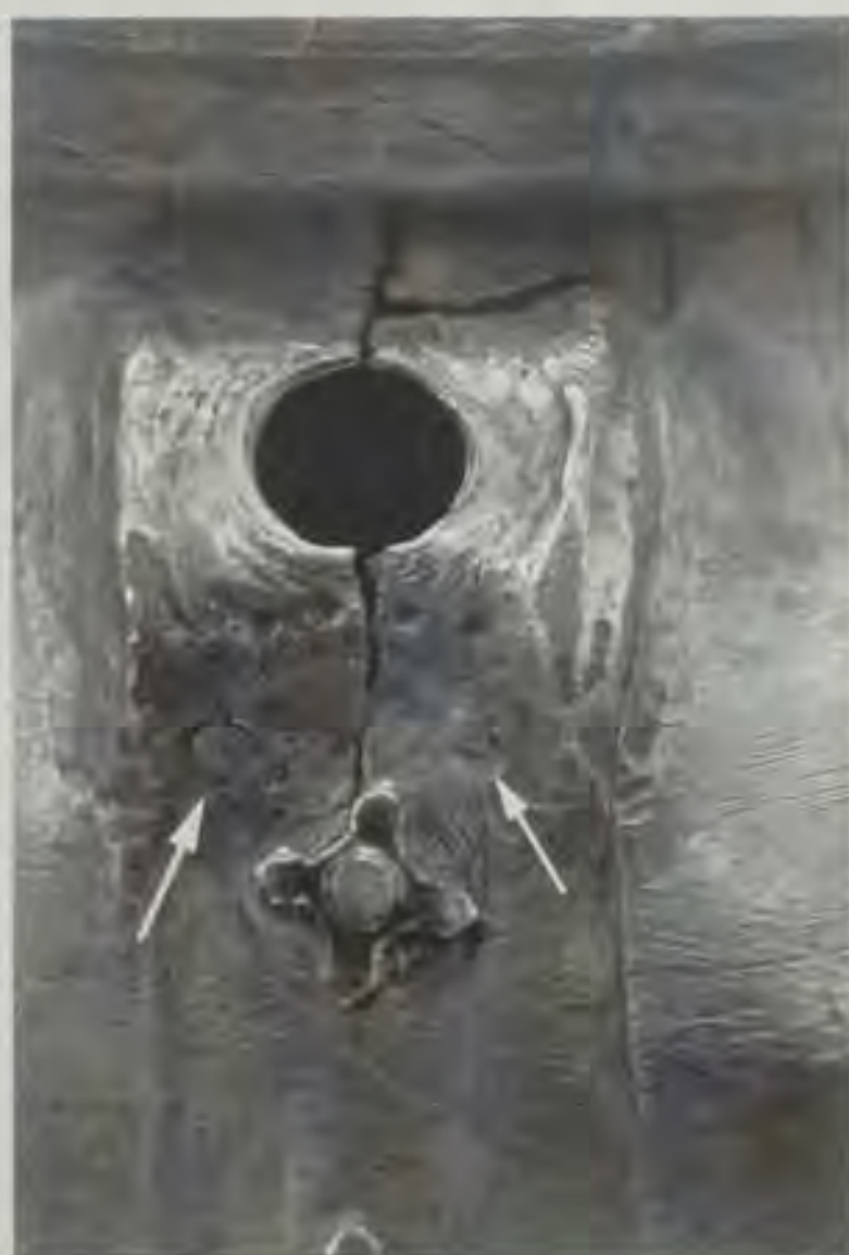
3a Detail of the underside of the stand, showing a crack that occurred where the sections were originally soldered together. The nuts are later additions to hold the armori-als. The two small pin-like circles are the cut-off remnants of the original wires that held the cast sections together during the soldering operation (as seen in 3b).
