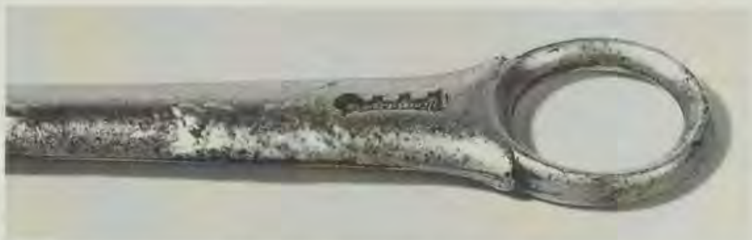
2 Skewer showing parting of the edge seam and the resultant blistering.
