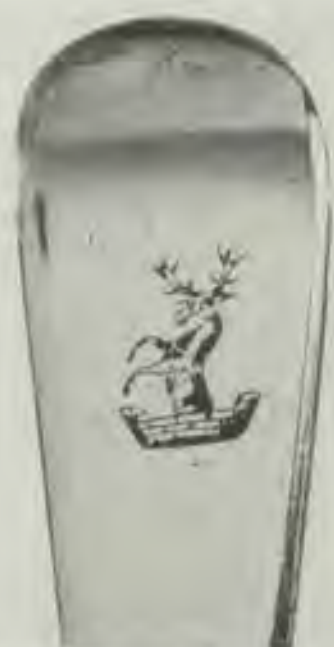
3 Engraved crest on fiddle pattern flatware. The silver foil has peeled away at the engraving.
