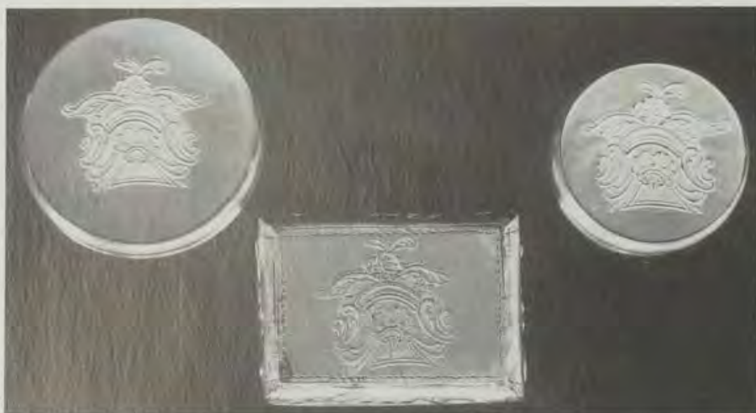
5 Three plated boxes with the same design die-stamped on the base. The rectangular example is the base of the box shown bottom centre in [3].
