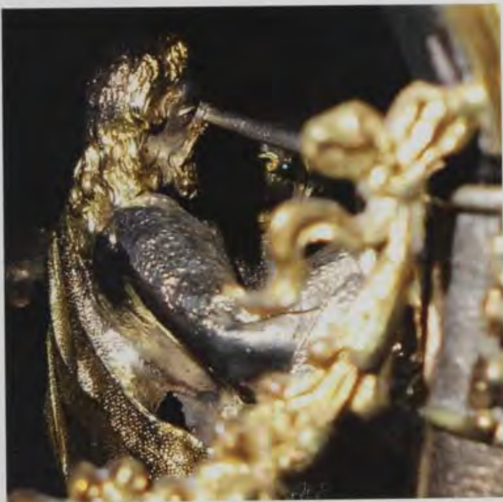
Fig 20: The Gilbert clock [Fig 5], detail of solder points to the back of the figure with a telescope (© The Rosalinde and Arthur Gilbert Collection on loan to the Victoria and Albert Museum, London)
