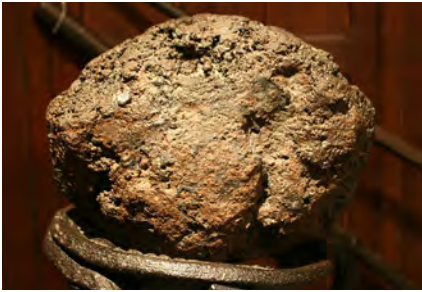
FIG 8 — Ball of Osmond iron [see note 25] (GNU Free Documentation License: courtesy of the Museum of Burg Altena. GFDL)
